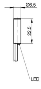
Inductive Sensors BES 516-371-SA 10-PU D6.5 x 22.5 normally-open Sn=1,5mm shielded
